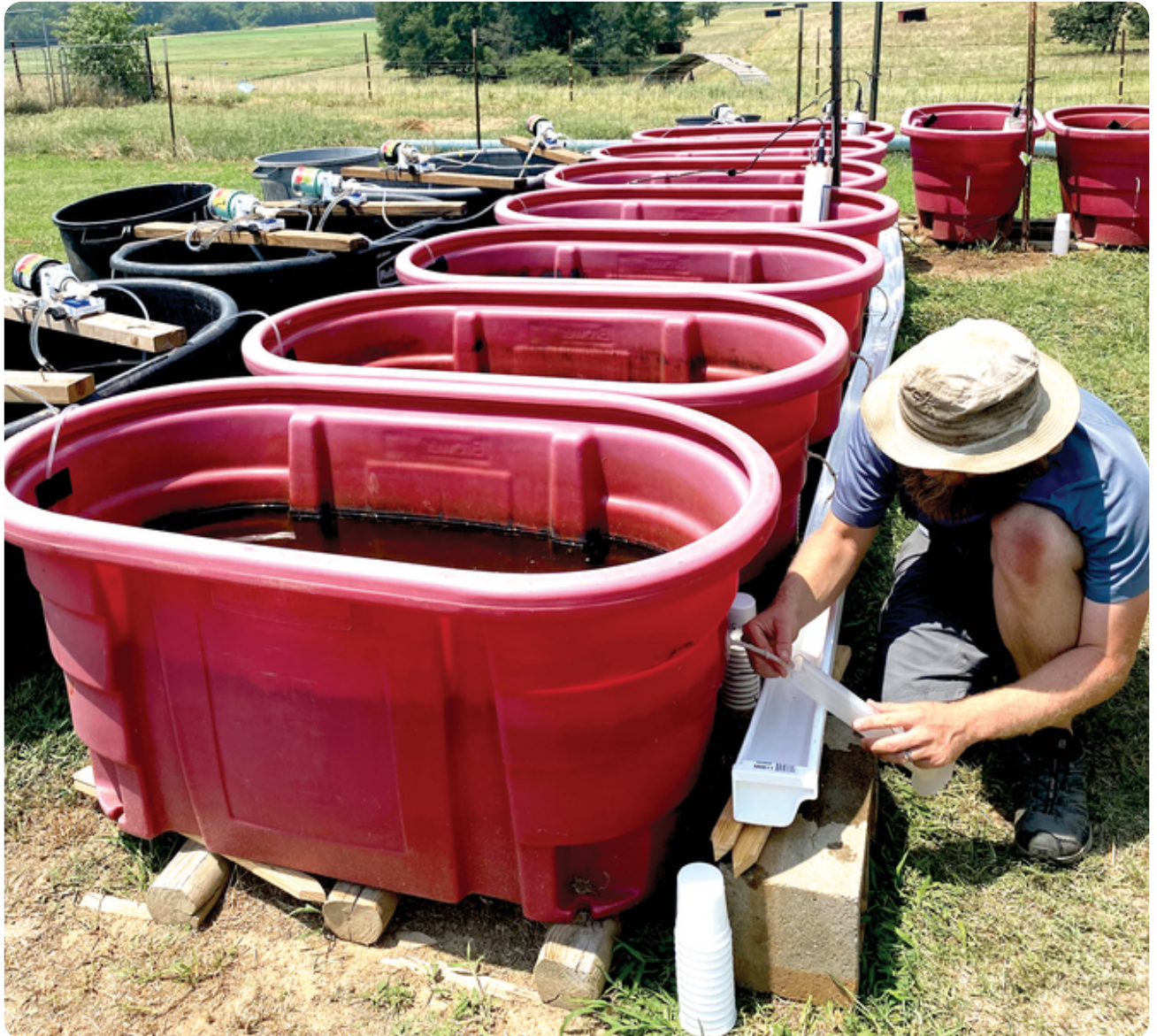
The experimental setup for testing the nutrient removal potential of woodchip bioditch reactors at the Arkansas State University Farm Complex in Jonesboro, AK. Photo by Jerry Farris.
