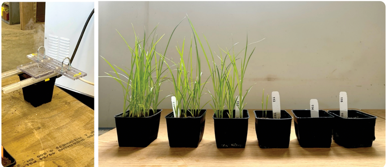
Figure 1. Pulse electric field (PEF) application in a pot study with yellow nutsedge tubers (left). The PEF energy quickly warms the soil; notice the water vapor. Yellow nutsedge plants 28 days after treatment with increasing rates of pulse electric field (right). Rates of PEF application were (l to r) 0, 15, 30, 60, 125, and 250 J/cm 3 .
