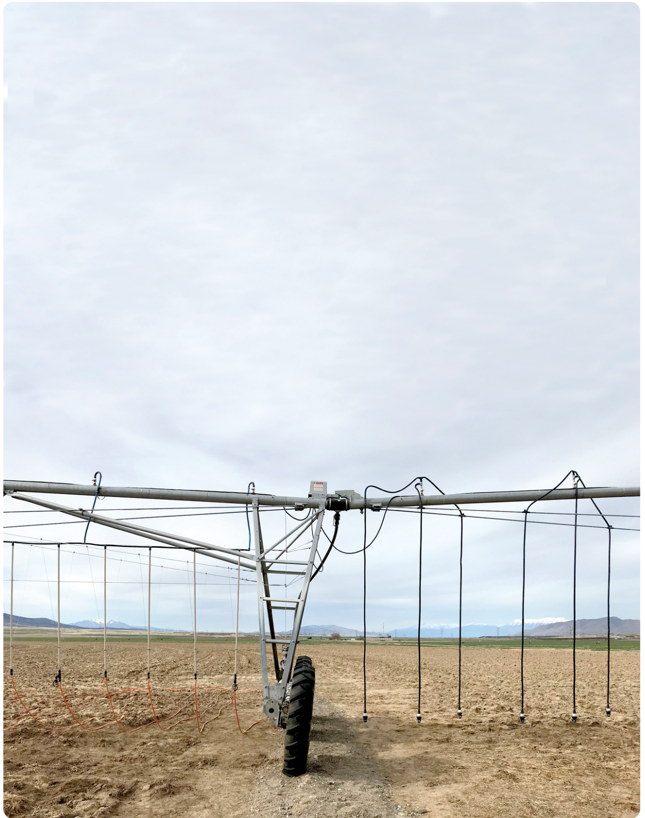
The low-elevation precision application (LEPA) sprinklers on the right were compared with mobile drip irrigation (MDI) on the left during a silage corn trial near Elberta, UT. Photo by Matt Yost.
