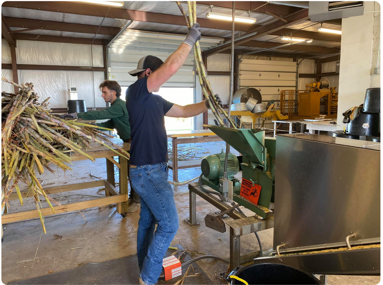
Blanchard passes whole sugarcane stalk samples through a shredder so the samples can be analyzed for sucrose content traits. Photo courtesy of Brayden Blanchard.
