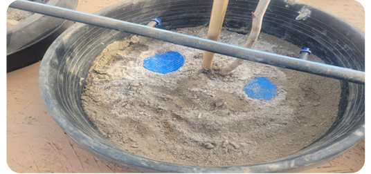
Figure 1. In a greenhouse experiment, pistachio trees were grown in a 10-gallon pot with drip irrigation and sap and stem diameter sensors.
