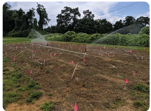
A field of thiamethoxam-coated soybeans in the study is irrigated with sprinklers. The plastic tubes represent the sampling ports for the soil water samplers to measure subsoil leaching. Photo by Ben Morrison.
