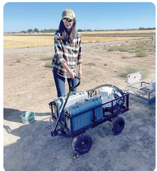
Abigail Baxter with a LI-COR unit that measures greenhouse gas emissions at the USDA-ARS Northwest Irrigation and Soils Research site in Kimberly, ID.
